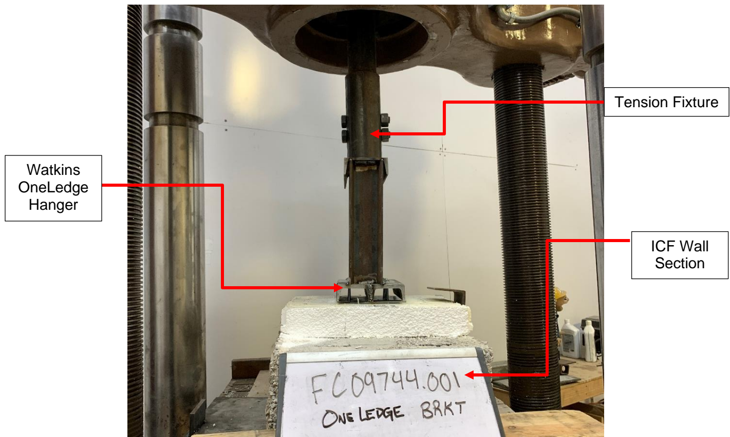
Figure 1. Pullout Resistance Test – Watkins OneLedge Hanger
